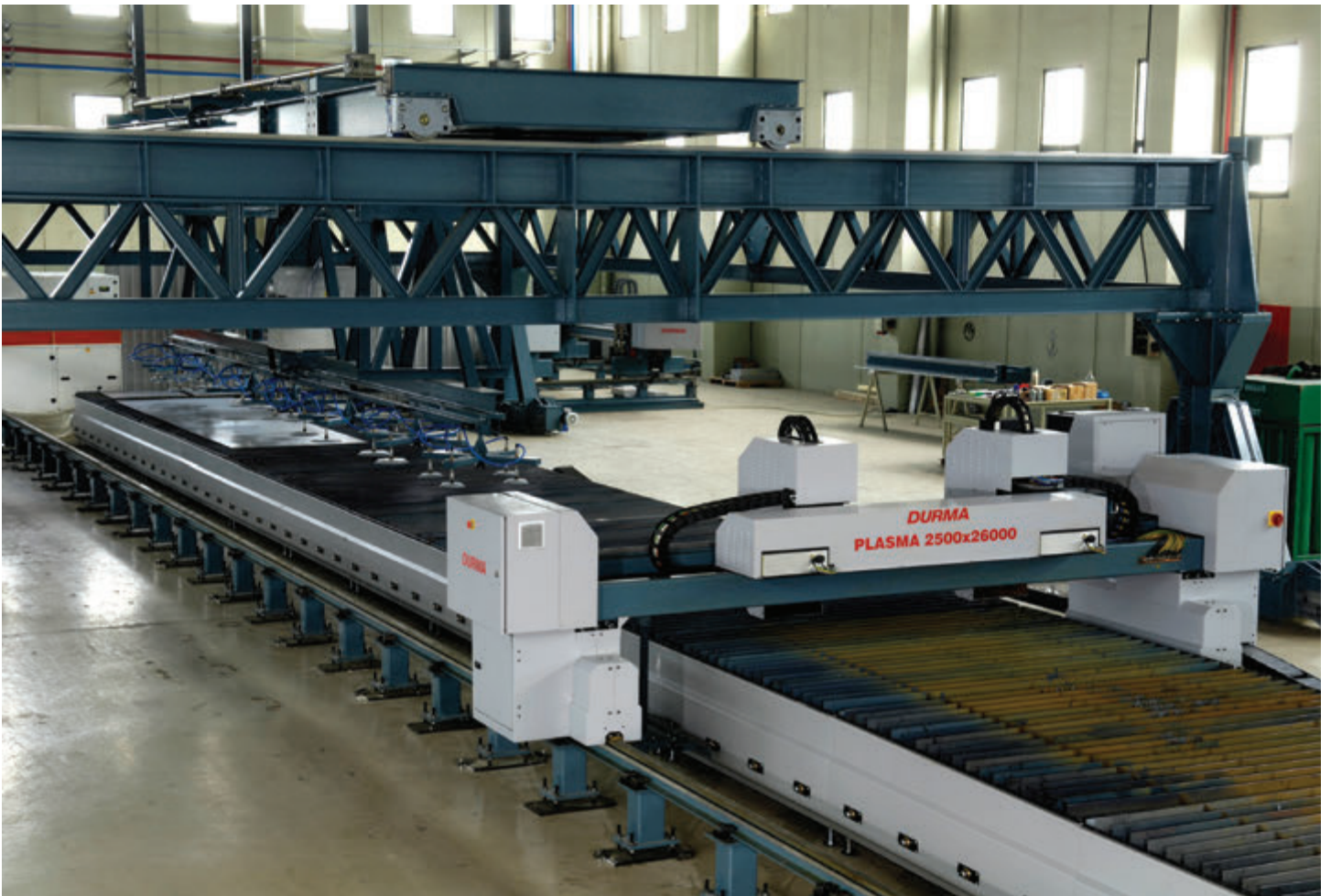
Plasma Cutting Machine with loading unloading system
